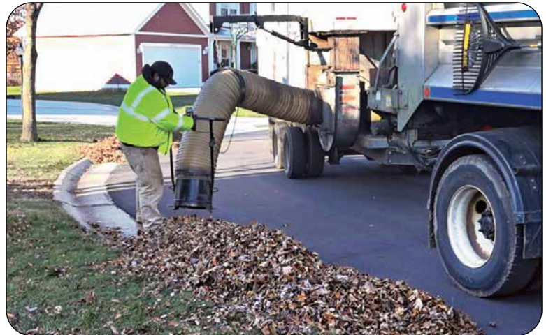
The image above shows how crews use a vacuum to collect loose leaves. Please follow the guidelines to the left to help prevent damage to the leaf vacuum and to make collection as effective as possible for all.
